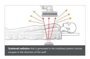
The variable opening of the drape, which can be placed on the patient exactly in line with the useful radiation zone, significantly reduces the scattered radiation. A classic example of application is ERCP\* but, in principle, a large number of other areas of application in which work is carried out with a fixed beam direction are possible.
